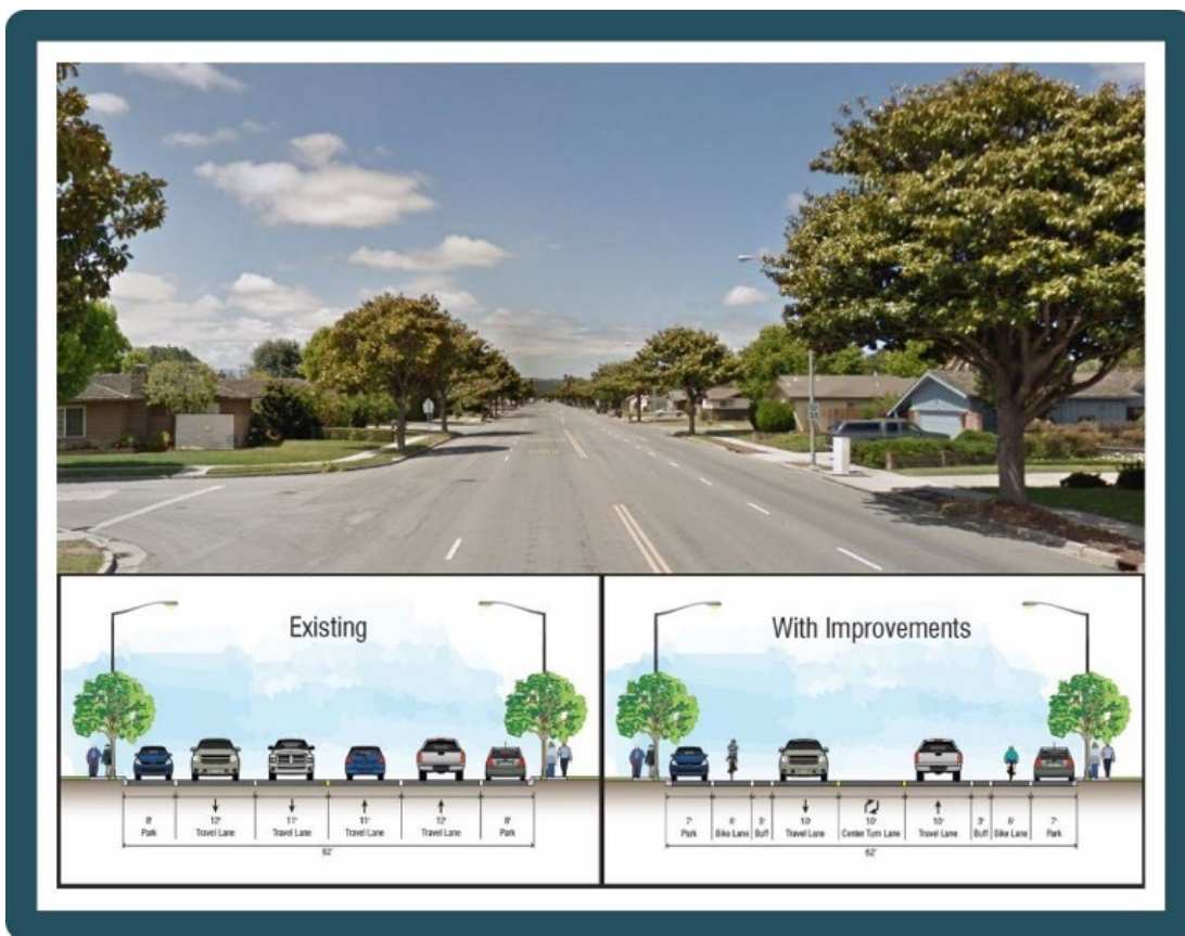
Figure 1: Roadway Configuration Before and After the improvements
