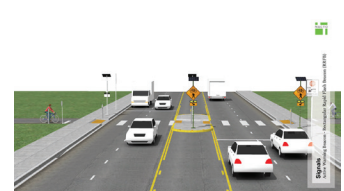
Rectangular Rapid Flashing Beacons
